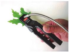
Our leaf clip bundle is specifically designed for leaf reflectance measurements. It features a separate tungsten halogen illuminator (ILM-105) to keep heat away from leaves during measurements to prevent burnout. An integral swing-away reflectance panel provides easy reference measurements
