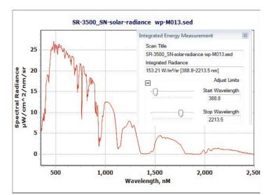
The full range SR-3500 was used to measure outdoor solar radiance using a 4° lens foreoptic and white reflectance panel. Pull down menus allow for easy calculation of integrated energy measurement over userdefinable boundary wavelengths .
