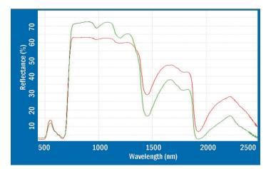
This scan was taken with an SR-3500 in the field using the leaf clip bundle accessory package. The red trace is acer saccharum and the green is rhododendron decorum. The leaf clip bundle option includes an ILM-105 fiber optic illumination module fitted with a one meter fiber optic bifurcated cable.
